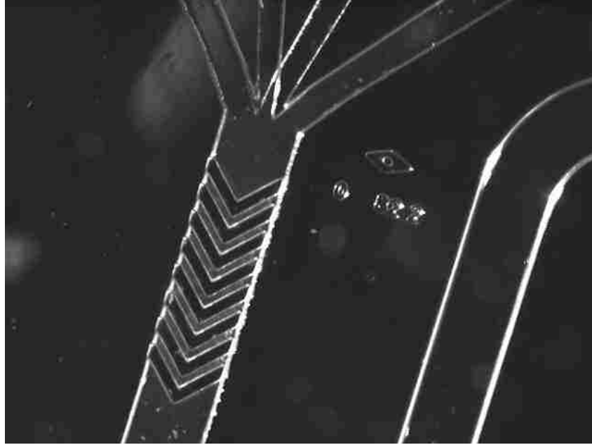
Figure 50: Image of an assembled SFD. Alignment of the PDMS layers is within a few \mu\text{m} of design, despite the material flexibility.
